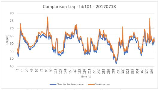
Figure 3: Broad band check (by using road traffic noise), considering 7 minutes as measurement time period – Time history of sound pressure levels, in terms of LAeq,1s [dB(A)].
