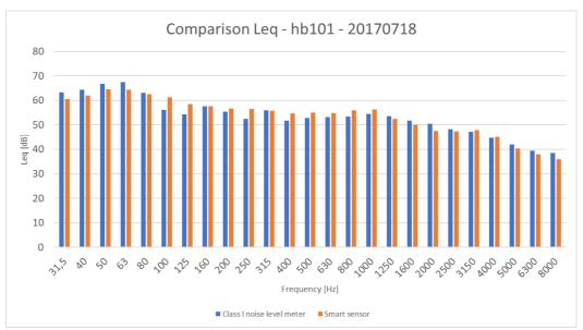
Figure 4: Broad band check (by using road traffic noise), considering 7 minutes as measurement time period – One third octave band sound pressure levels, in terms of Leq,10' [dB].
