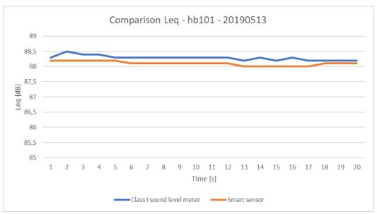
Figure 5: Broad band check (by using an electroacoustic source and a pink noise signal), considering 30 seconds as measurement time period – Time history of sound pressure levels, in terms of LAeq,1s [dB(A)].
