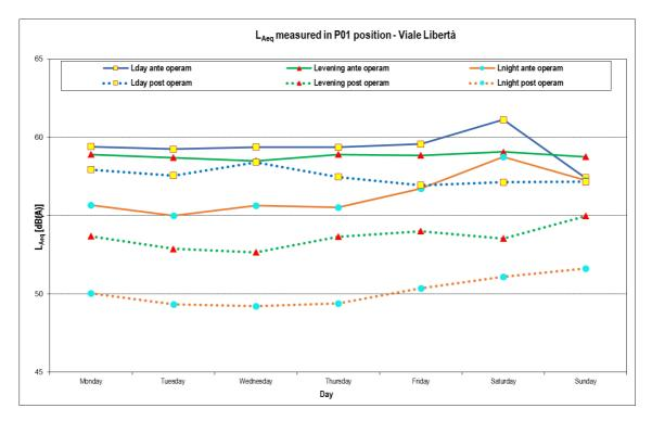
Figure 1 – Comparison of noise levels measured with class I instruments in winter in the ante- and post-operam scenarios.
