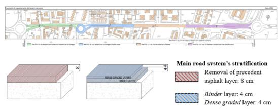
Figure 2. Detail of the design of low-noise pavement in Viale Libertà - Monza.
