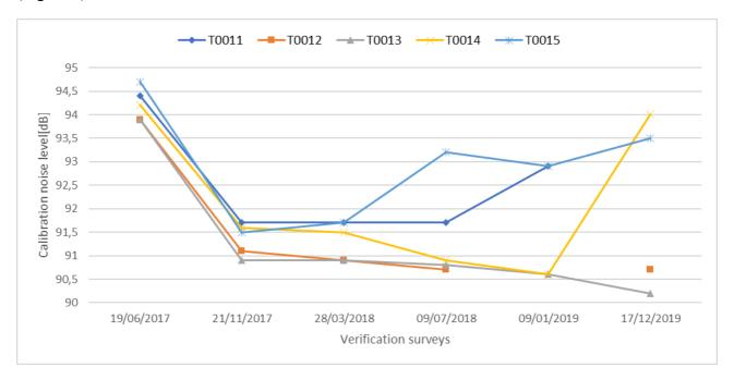
Figure 1: 1 kHz calibration check – MEMs sensors placed on poles.
