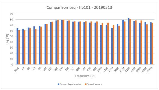
Figure 6: Broad band check (by using an electroacoustic source and a pink noise signal), considering 30 seconds as measurement time period – One third octave band sound pressure levels, in terms of Leq,30s [dB].
