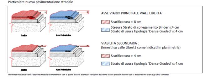
Figure 2 – Detail of the new soundproofing road pavement
