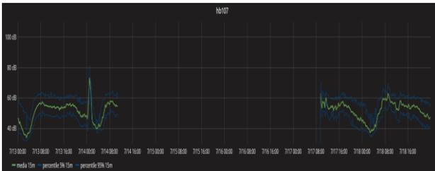
Figure 4. Breakage of microphone put in evidence by the signal interruption shown by the time history of sound pressure levels.
