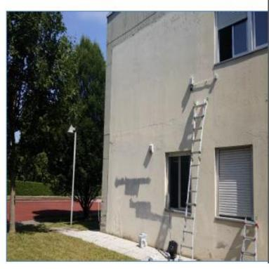
Monitoring stations located on streetlight or on façade, height 4 m; power supply: solar panel and energy network.
