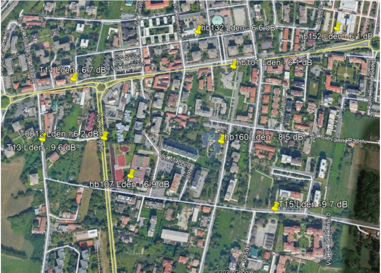
Figure 3: Noise levels reduction (Lden) measured by each smart sensor between the II week of January 2020 and the III week of March 2020.
