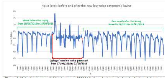
Figure 5. Noise levels recorded by the sensor HC101 before, during and after the laying of the new road surface
