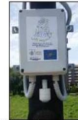
Figure 2: Smart-noise monitoring system
