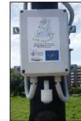
Figure 2: Smart-noise monitoring system
