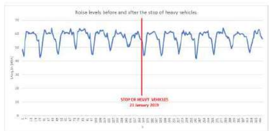
Figure 6. Noise levels recorded by the sensor HC101 before and after the stop of heavy vehicles
