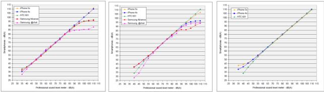
Figures 17-18-19. On the left, comparison results, using the internal microphone of smartphones; the central figure shows the results using the original headphones of the smartphones. On the right, comparison using the MicW microphone plugged into the smartphones. Source: [23]
