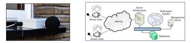
Figures 5-6. On the left, a sensor node, placed on a windowsill of a building and, on the right, the scheme of the smart sound monitoring sensor network architecture. Source: [10]
