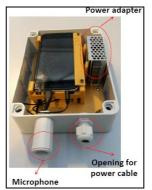
Figures 20-21. Hardware set-up for outdoor noise measurements, using smartphones. Source: [24]
