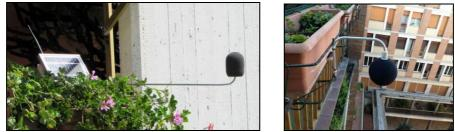
Figures 7-8. On the left, Zigbee transmitter with a solar panel and a microphone installed on a balcony (2011). Source: [12]; On the right, microphone of a monitoring station for anthropic noise assessment. Source: [14]
