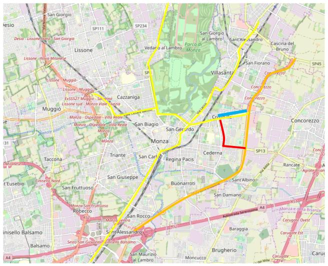
Figure 2 – Heavy vehicle traffic limitation: the forbidden route in blue, the possible alternative route in red
