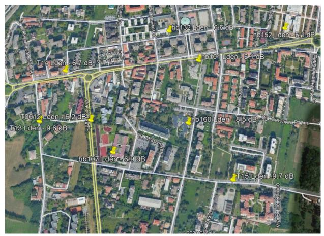
Figure 3: Noise levels reduction (Lden) measured by each smart sensor between the II week of January 2020 and the III week of March 2020.
