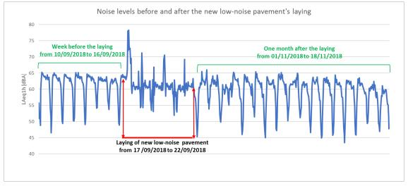
Figure 2 - Noise levels recorded by the hb101 sensor before, during and after laying the new paving.
