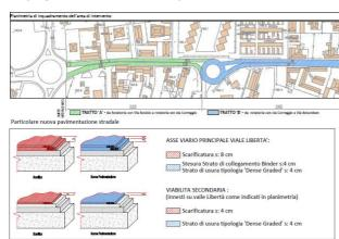
With the aim to reducing noise pollution in the pilot area of Viale Libertà in Monza, two main interventions were designed and implemented: the drafting of a new low-noise asphalt and the limitation of traffic to heavy vehicles.
